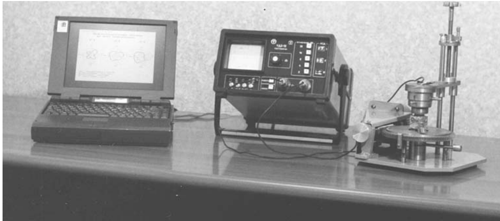
Fig. 4.11. General view of the automated acoustopolariscope with ultrasonic device and computer (The authors of this construction are Golovataya O.S, Gorbatshevich F.F.)
