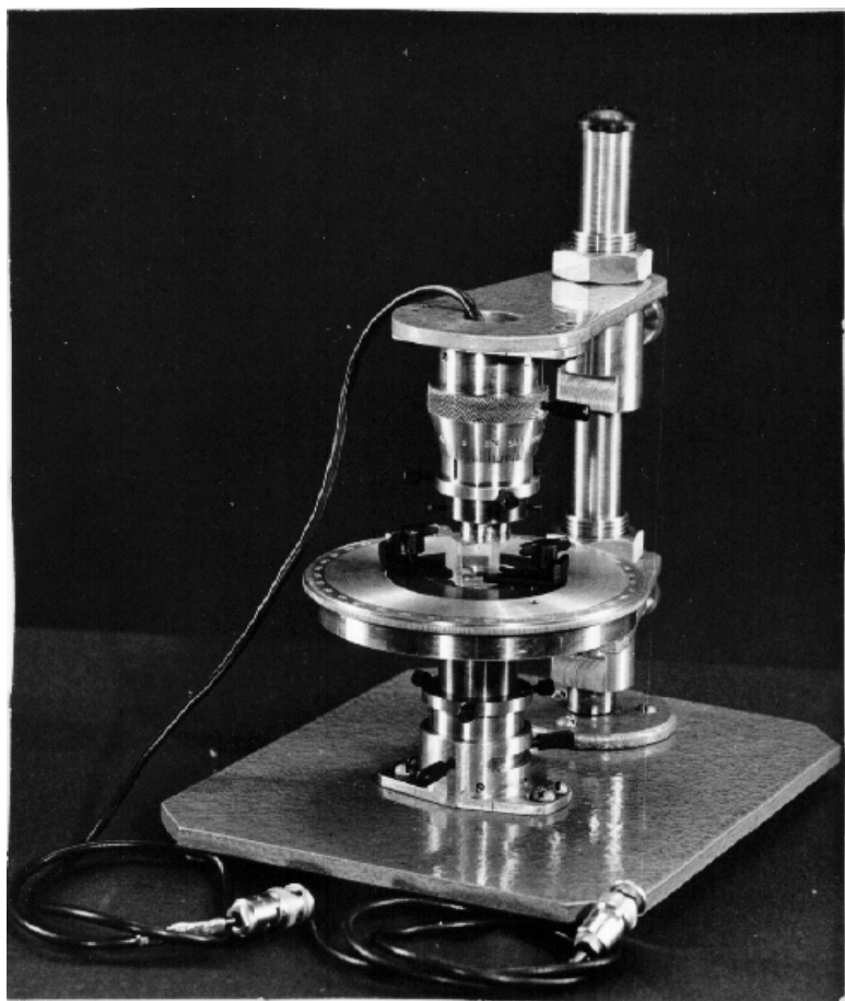
Fig. 4.9. General view of acoustopolariscope with rotating platform (Patent N 1281993, USSR). One pole type.
